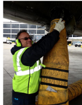
American ORD Fleet Service Clerk George Echevarria connects the pre-conditioned air (PCA) hose to an aircraft. Using available ground power and PCA equipment instead of the APU saves jet fuel and eliminates more CO 2 emissions.
